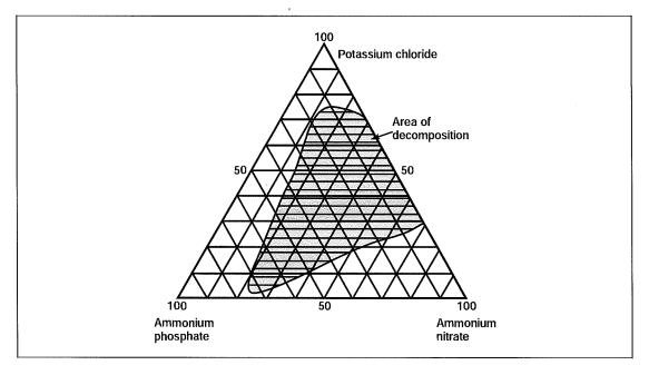
Fig. 2. Area of Fuse-type Decomposition in Mixtures of Ammonium Nitrate, Ammonium Sulfate, and Potassium Chloride.
