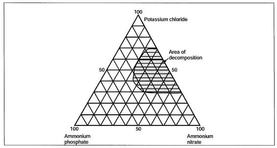
Fig. 1. Area of Fuse-type Decomposition in Mixtures of Ammonium Nitrate, Ammonium Phosphate and Potassium Chloride.
