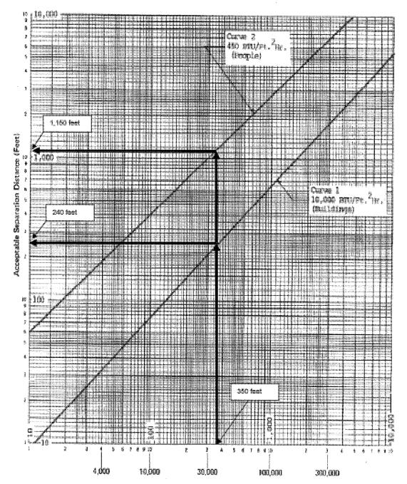
Figure 2: Acceptable Separation Distance Calculation for Buildings and People (Thermal Radiation)
