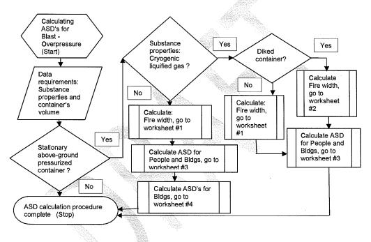
Proceed to calculate the fire width, using Worksheet 1. Use Worksheet 1 because the dike area on a pressurized container does not have any effect on the ASD calculations. Following with the procedure, the volume of the container (30,000 gallons) is plotted in the x-axis toward the line graph, making an intersection with the line graph. This intersection point is then plotted toward the y-axis, providing the fire width (see figure 1). The fire width was determined to be 350 feet.
