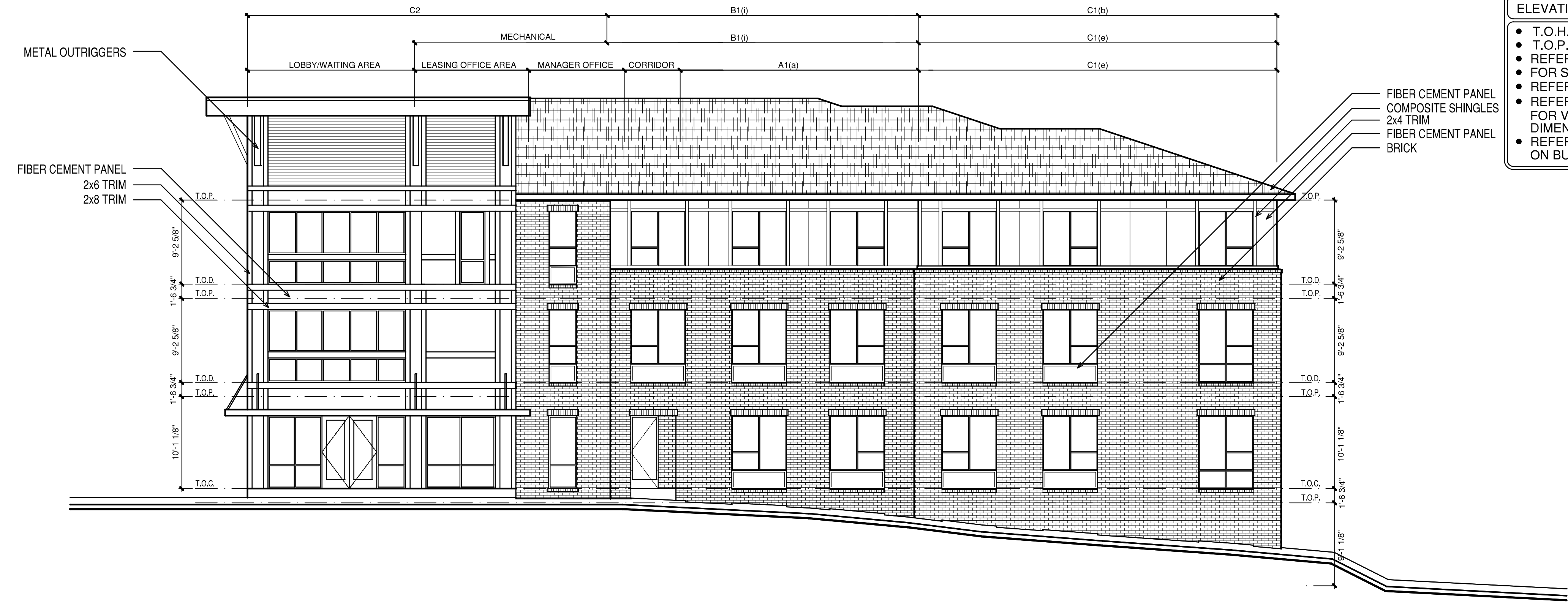
2 ELEVATION - BUILDING B - EAST SCALE: 1/8" = 1'-0"
