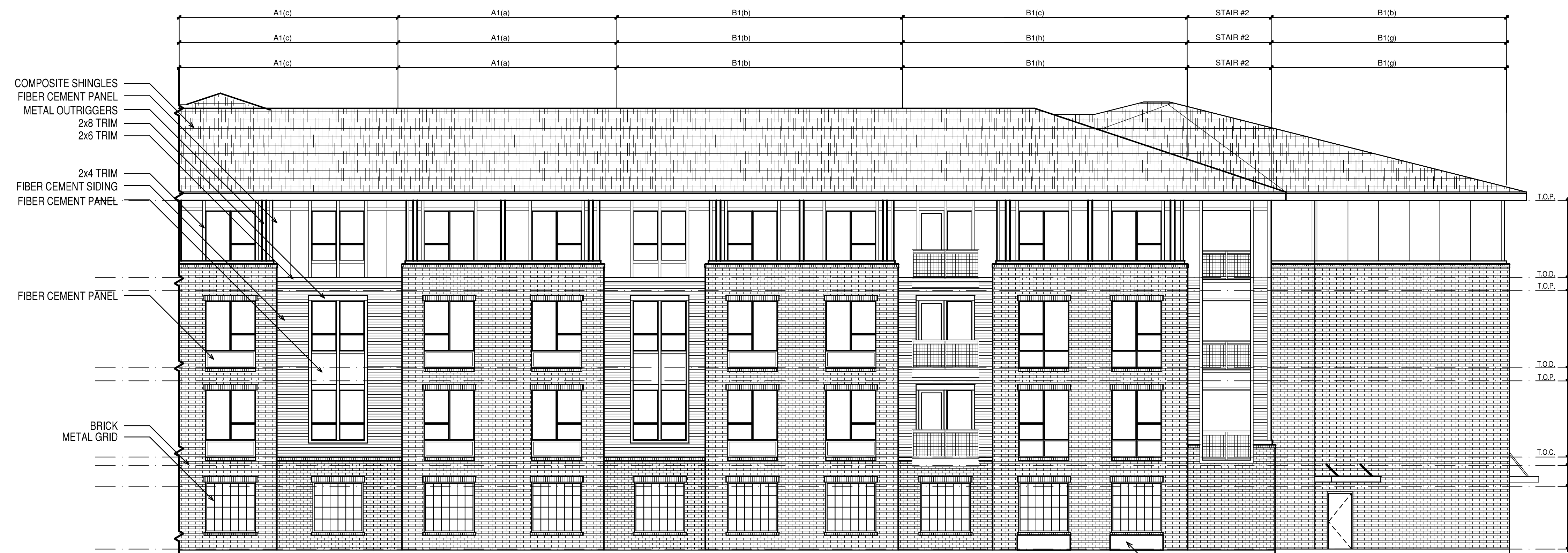
2 ELEVATION - BUILDING A - WEST SCALE: 1/8" - 1'-0"
