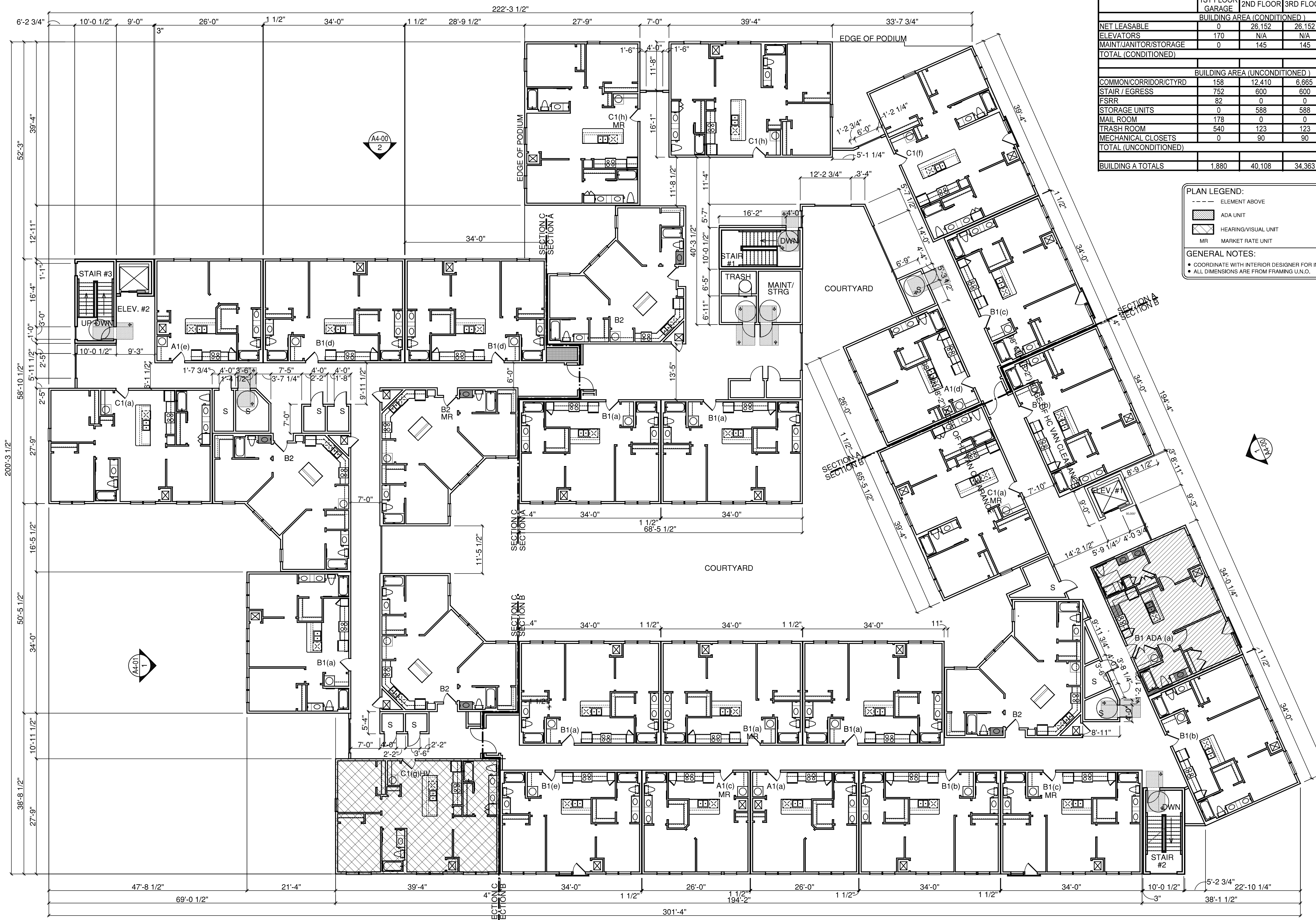
1 FLOOR PLAN - BUILDING A - FOURTH FLOOR SCALE: 3/32" = 1'-0"
