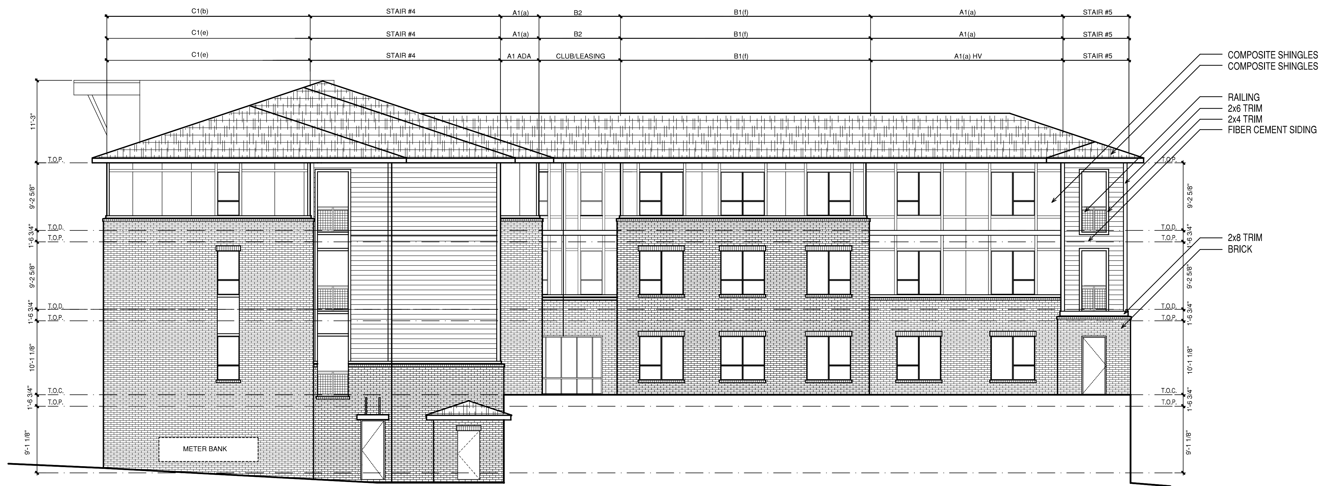
2 ELEVATION - BUILDING B - WEST SCALE: 1/8" = 1'-0"
