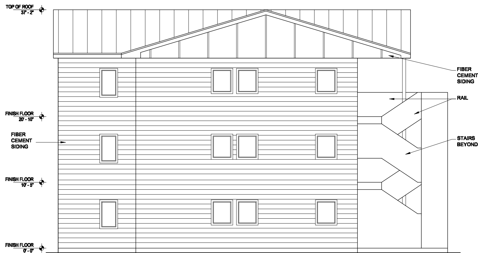
LEFT SIDE ELEVATION BUILDINGS A & C
