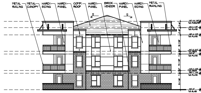
1. BUILDING TYPE 2 EXTERIOR ELEVATION
