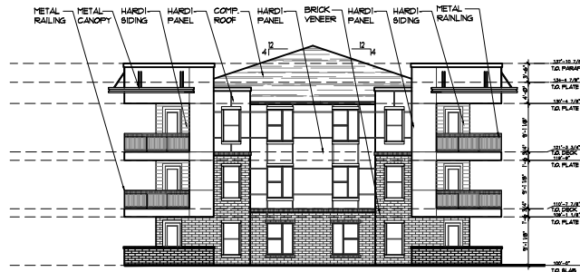
2. BUILDING TYPE 3 EXTERIOR ELEVATION
